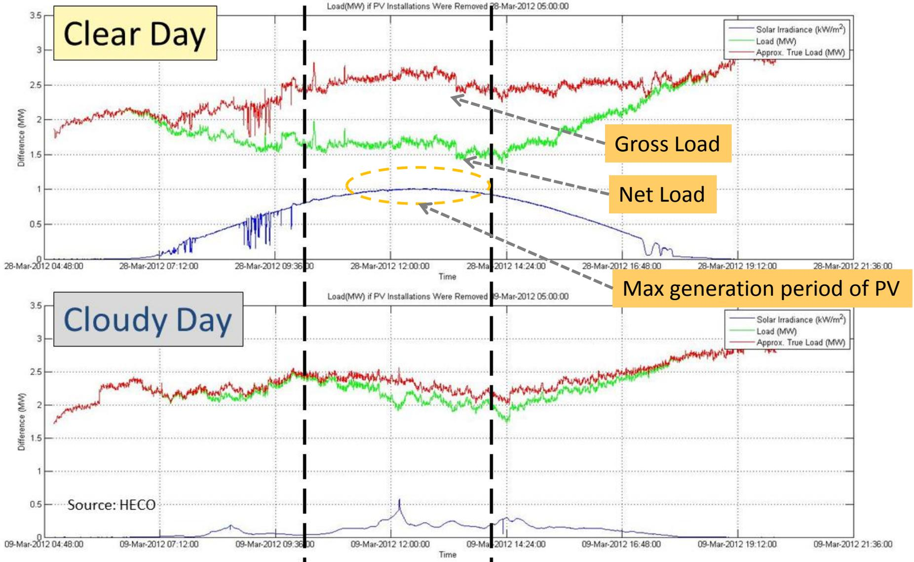
Greatest Feeder PV to Load Variation Between 10 AM and 2 PM
